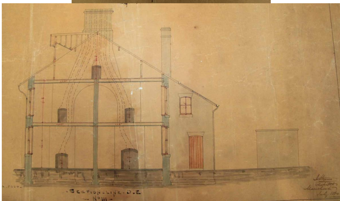
Fig 5 Cross-sections of proposed houses, showing one with transverse stair (13-18 Heol y Dwr / Water Street) and one with an attic storey and overhanging eaves (19-24 Heol y Dwr / Water Street), drawn by James Stevens of Manchester. (© Talyllyn Railway Archives)
