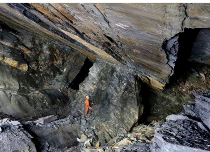
Figure 3.9. Underground at Maenofferen in Ffestiniog (Component Part 5) – this former working chamber is one of the few surviving examples of the oldest method of supporting a roof in a slate mine, by leaving a column of slate in place.
