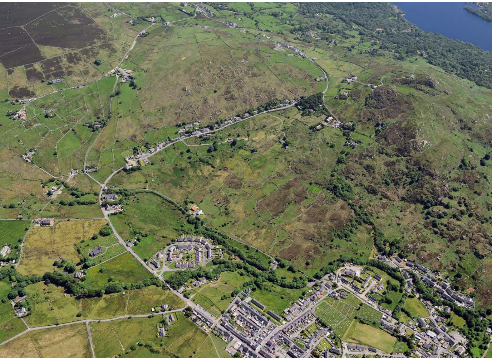
Figure 2.45. Both the slate road through the village of Deiniolen and the 1825 Dinorwig Slate Quarry Railroad are evident in this aerial view. The Railroad can be traced as a tree-grown formation making its way down the slope on the right of the photograph.
