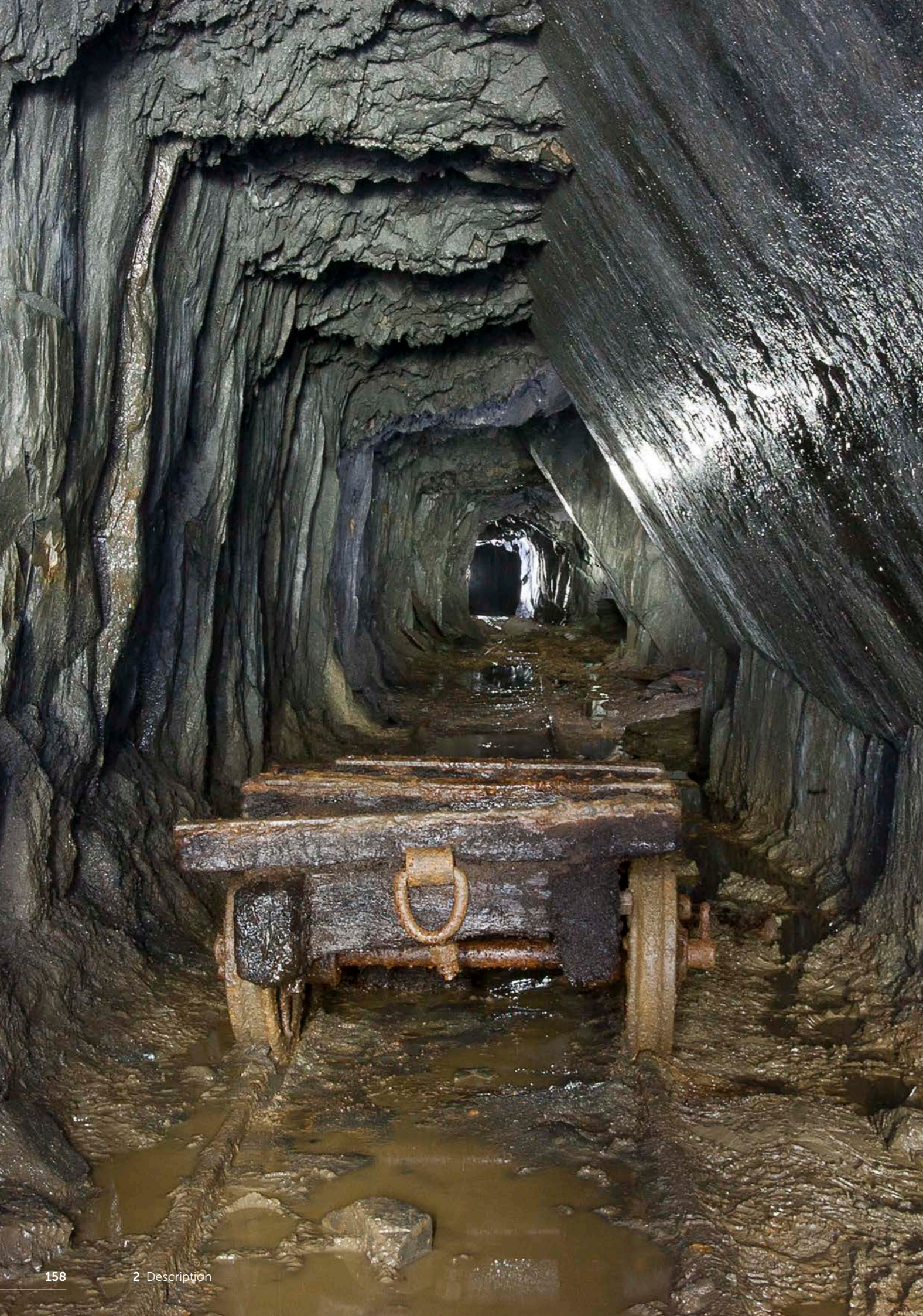
Figure 2.108. Much of the underground workings at Bryneglwys is above the water table and accessible to specialists. They preserve equipment from various phases of the quarry's period of operation such as this flat wagon. See Figure 2.10.
