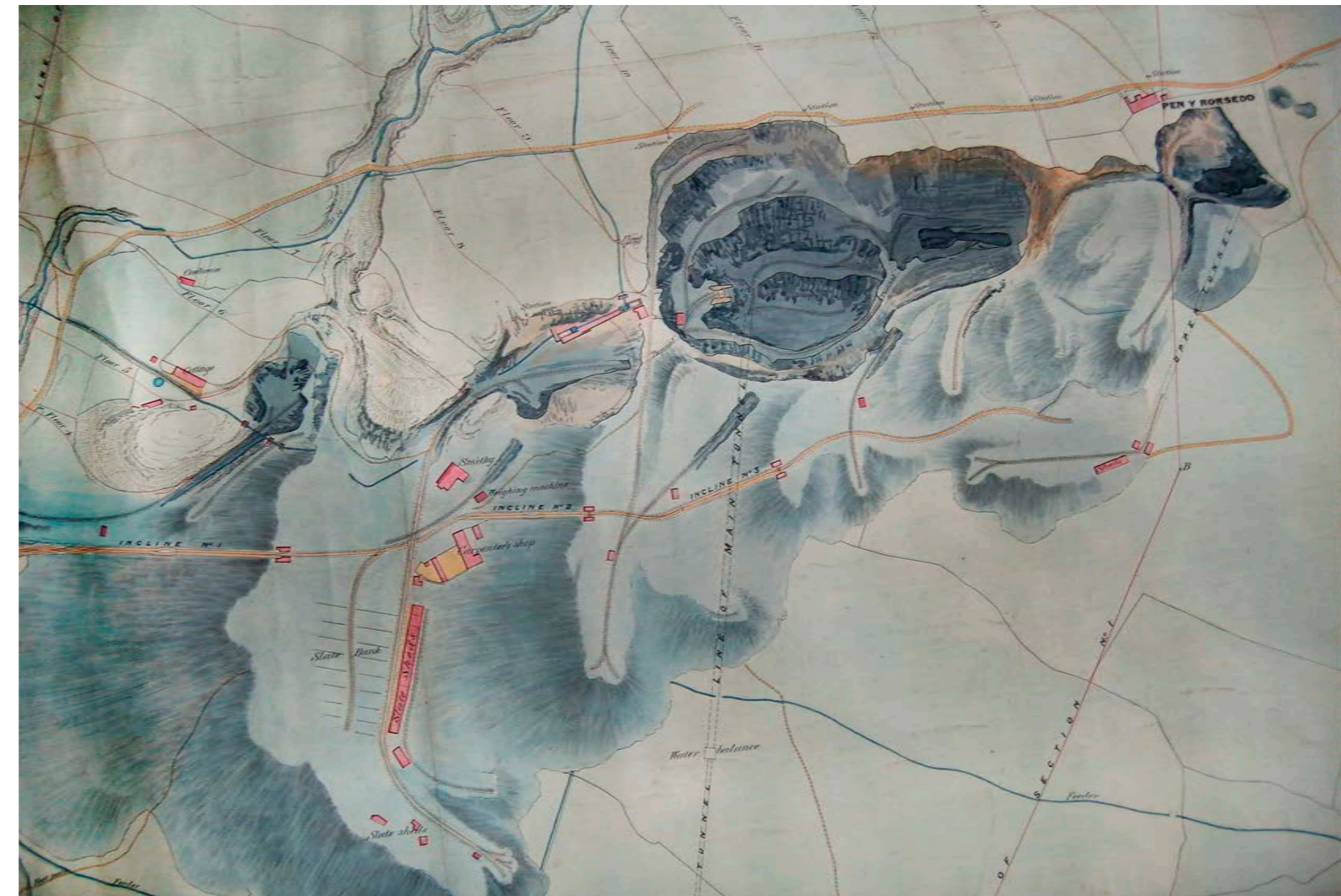
Figure 2.154. Though Bryneglwys Slate Quarry is the only site in The Slate Landscape of Northwest Wales where the technology of the water-driven chain incline can still be seen in situ (Element 6.1), sources such as this map of 1862 show it was first evolved at Pen yr Orsedd Slate Quarry in Component Part 3. It was exported to Bryneglwys by Nantlle men. Surviving archaeology and documentary sources such as this are important in establishing how particular technologies functioned and were disseminated. A change of management brought in Ffestiniog quarrymen shortly afterwards; they introduced their own characteristic way of working the rock – from underground chambers.
