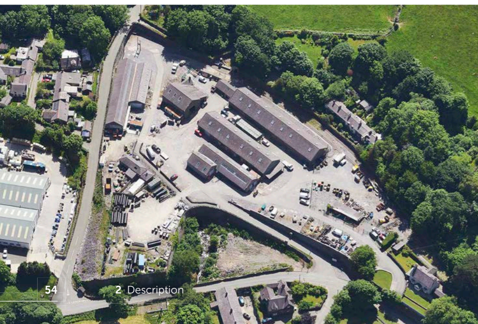
Figure 2.16. This aerial view of the Felin Fawr slab mill and engineering complex shows how the two slab-mills and their associated engineering complex were constructed above a culvert carrying the stream that powered the waterwheels. Also evident are a foundry, the course of the railway, locomotive sheds and workers' housing. The buildings are now operated by a local business, and have been conserved.
