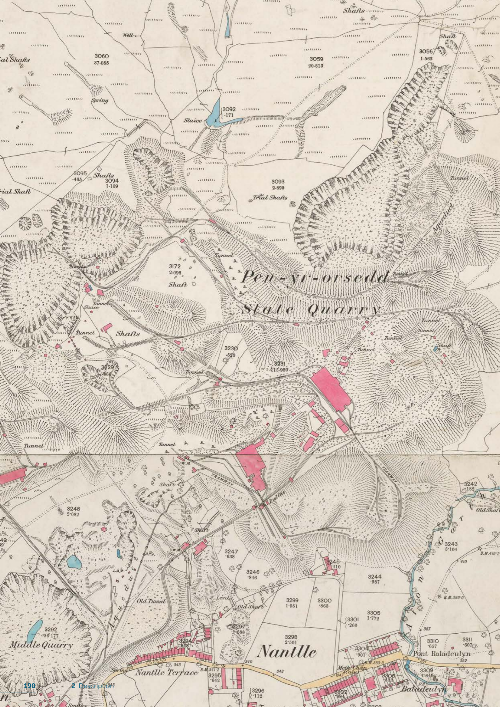
Figure 2.139. The 1889 25 inch to 1 mile ordnance survey map of the Pen yr Orsedd Slate Quarry (Element 3.7) illustrates how the rock was worked in the Nantlle Valley. Rubble and blocks are raised by means of aerial ropeways spanning the pits, then moved by locomotive respectively to the tip-ends for dumping, and to mills to be mechanically sawn and then split by hand.
