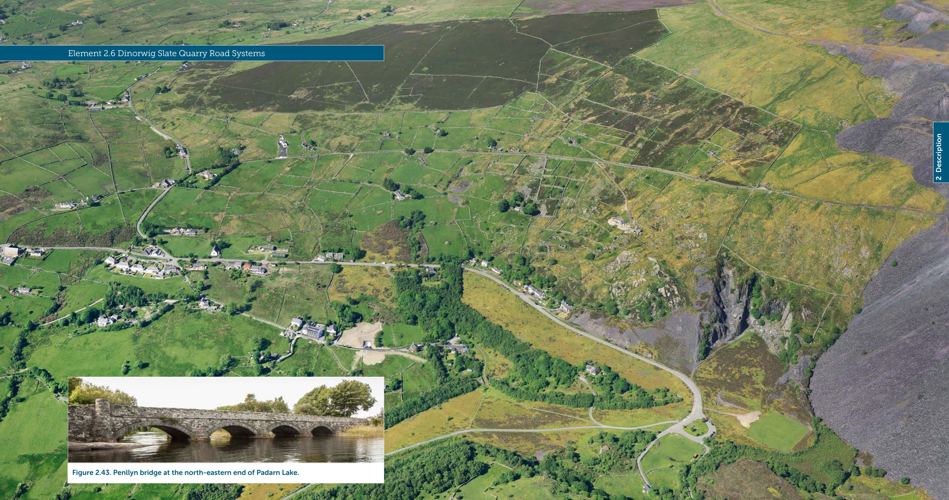
Figure 2.44. The uppermost road here led to the upper 'Garret' galleries in the quarry. It was designed and built by Thomas Telford's assistant William Alexander Provis in the 1820s, part of the pre-railway network that transported Dinorwig slates to the sea. It makes its way through the small plots of land leased to quarry families to provide for themselves by building homes and growing food.
