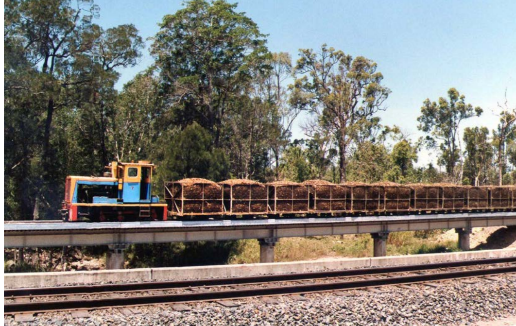
Figure 3.36. Diesel traction replaced steam on Queensland's 0.6m gauge sugar cane railways by the 1970s. Here a train makes its way over a bridge at Mackay, parallel to the North Coast Railway which runs on 1.067m gauge.
