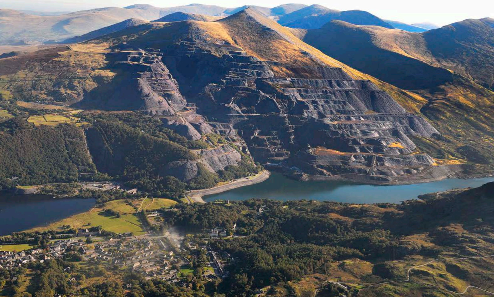
Figure 2.32. Dinorwig Slate Quarry is reflected in the waters of Peris Lake. The massive system of inclined planes shows how these transport systems made ingenious use of topography to ensure internal movement of slate rock. Locomotive-worked railway systems ran along each of the stepped galleries to the massive tips of waste rock.
