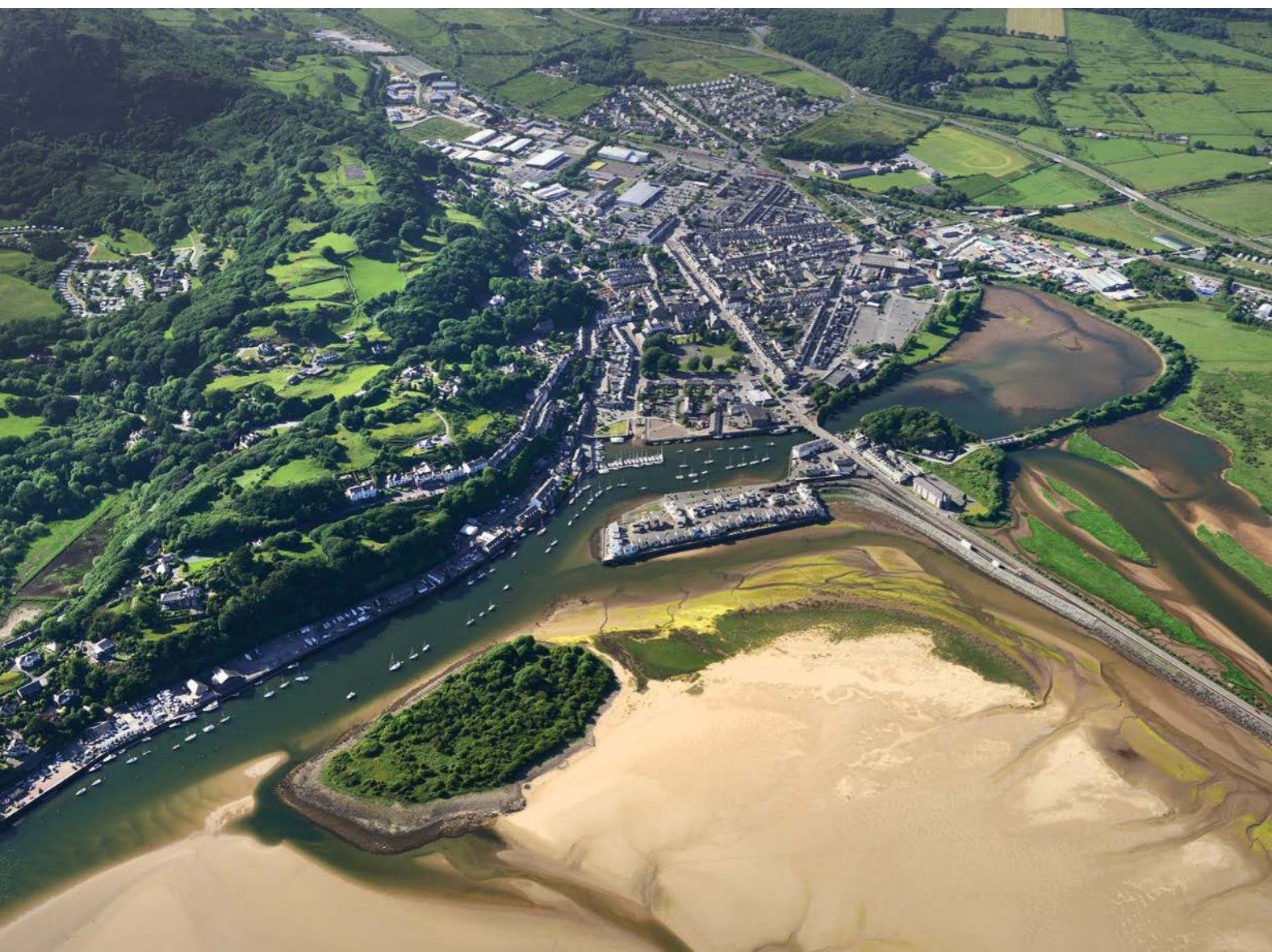
Figure 2.103. The last stage of the journey from the quarries to the sea takes the Ffestiniog Railway over a sea-defence built in 1808-1811, shown here on the right. Diverting the Glaslyn River scoured out a harbour (left). The quays were built between 1824 and 1867 to facilitate the transfer of Ffestiniog slates, initially from small river-boats, later from the railway, to ocean-going sailing ships. The Ballast Bank (left foreground) is made up of stones discarded as ballast from slate-ships returning without a cargo. Porthmadog Harbour is widely used by pleasure craft.
